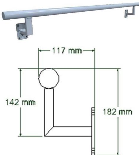
ABCO Wall Mounted Rails are designed and manufactured in Australia.
